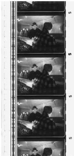
1.18 35mm is the standard theatrical film gauge. The sound track, a variable-area one (p. 00), runs down the left alongside the images.
