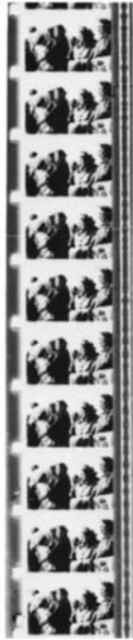
1.17 16mm film is used for both amateur and professional film work. A variable-area optical sound track (p. 00) runs down the right side.
