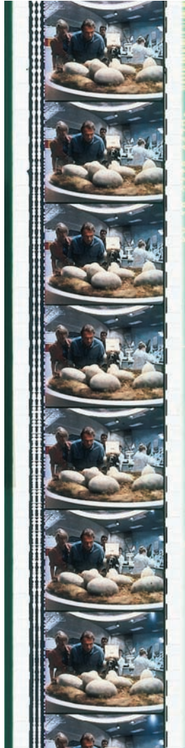
1.19 In this 35mm strip from Jurassic Park , note the optical stereophonic sound track (p. 00), encoded as two parallel squiggles. The stripe along the left edge, the Morse code–like dots between the stereophonic track and the picture area, and the speckled areas around the sprocket holds indicate that the print can also be run on various digital sound systems.
